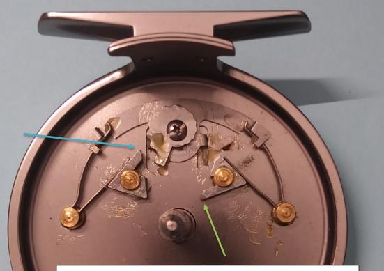
\*Set up to crank with left hand.
