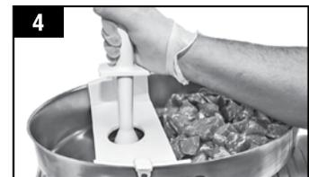
**WARNING! NEVER RUN GRINDER DRY WITHOUT MEAT! It can cause damage to the unit. Meat becomes a lubricant when passing through the grinder head. If you run out of meat, turn the grinder off immediately.**
