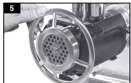
**DO NOT OVERTIGHTEN!** Over tightening adds pressure on the grinder assembly that will cause increased heat-generating friction in the grinder head and will stress the motor.
