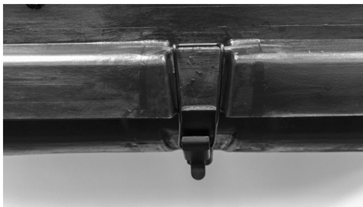
Place bale latch into closed and locked position
